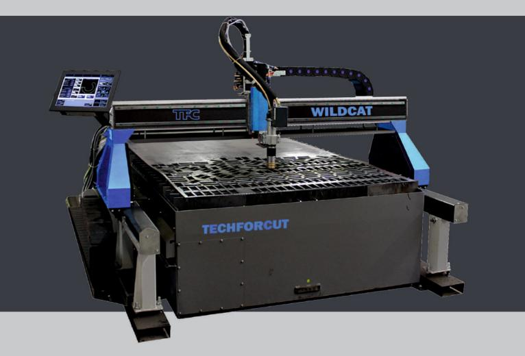
WILDCAT is the portal CNC cutting machine that combines gas and plasma cutting technology at a very reasonable price. It can be equipped with both standard air plasma and plasma for high precise cutting.
